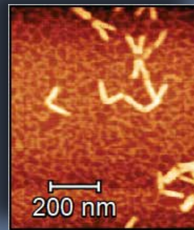
AFM topograph of DNA origami "tweezers," with individual DNA strands in background. Courtesy of Walter lab.
