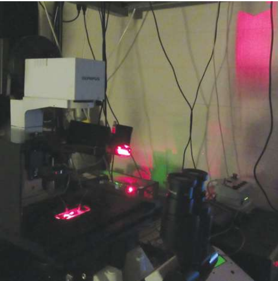
The Single Particle Tracker (SPT) microscope at the SMART Center, shown here, is being updated to meet evolving research needs. A suite of new components, including new cameras, lasers, temperature control for both sample heating and cooling, and microfluidic flow controls enable an array of multiplexed imaging techniques. Photo: Elisabeth Paymal
